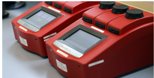
PCR cyclers for running three different PCR reactions in one machine.
