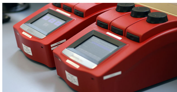
PCR cyclers for running three different PCR reactions in one machine.
